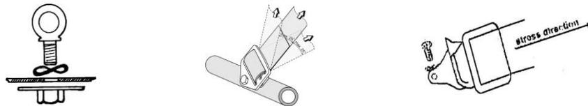
Lap belts must be positioned so that the mounting hardware through which the webbing passes is loaded in plane as the webbing passes through the seat and over the pelvis. Bolt-on brackets must be allowed to swivel and snap-on eye bolts must be aligned (using wavy washers) to allow directional loading.
