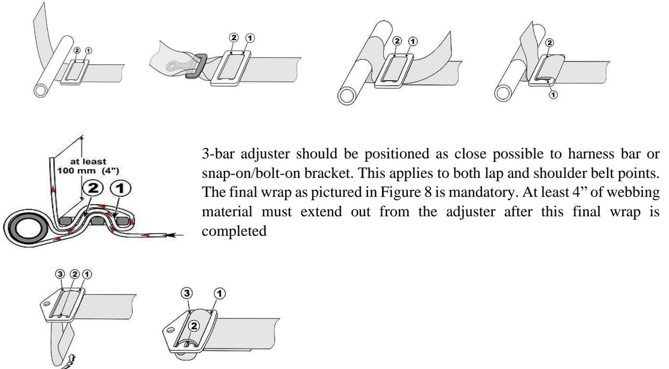
3-bar adjuster should be positioned as close possible to harness bar or snap-on/bolt-on bracket. This applies to both lap and shoulder belt points. The final wrap as pictured in Figure 8 is mandatory. At least 4” of webbing material must extend out from the adjuster after this final wrap is completed
